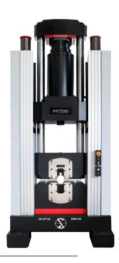
The DI-CP/V2 model, which is part of the PRO series, has been designed to perform tensile, compression, bend/flex and shear testing, with nominal capacity between 1500 and 2000 kN. Tension is always tested using the hydraulic grips, located in lower area, and compression in the upper test area.
