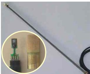
**type LFLT40** air temperature and rel. humidity sensor
