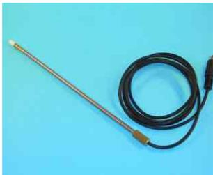
**type LFLT55 very thin** air temperature and rel. humidity sensor
