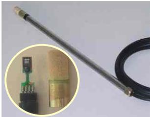
**type LFLT20** air temperature and rel. humidity sensor
