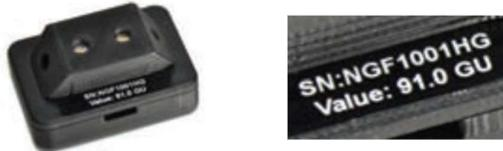
2. Attach tile to measurement head; for best performance place on a flat surface.
