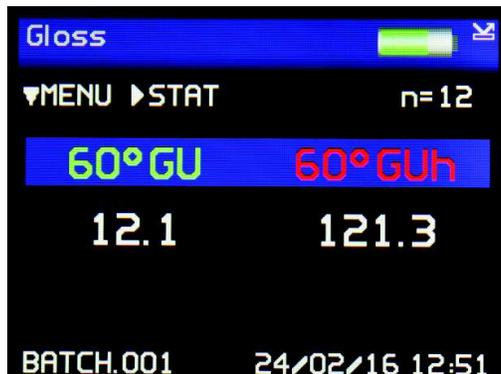
Pressing the Right button in the home screen will access the statistics screen for the current batch. Measurements can be taken whilst in this screen and the statistics will be updated.
