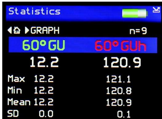
If the pass/fail feature is enabled, the colour of the angle header indicates if the last reading is within the user defined tolerances.
