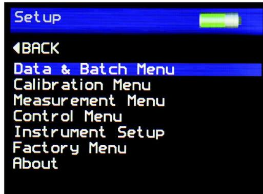
The Setup Screen is used to customise the instrument to the user's preference. Pressing the Up and Down buttons navigates through the options, pressing the Enter button selects that option.
