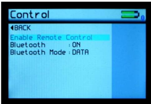
3. If the Bluetooth icon is not visible, enable it as detailed in Control Screen. Ensure that Bluetooth mode is set to either Data or Data+
