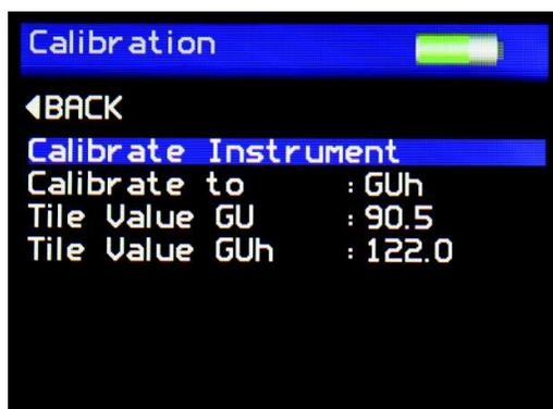
The Calibration Screen is used to setup the instrument calibration to the user's preference. Pressing the Up and Down buttons navigates through the options, pressing the Enter button selects that option.
