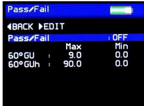
The pass/fail setup screen is used to enable/disable on screen pass/fail indication and set measurement criteria.
