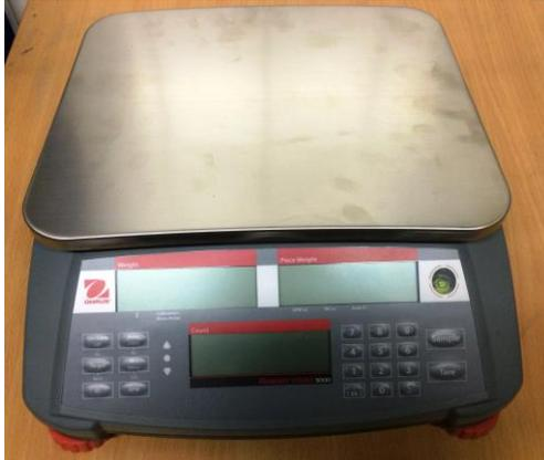
The Ohaus Ranger 3000 counting scale is designed to be the best compact counting scale in its class. It is a high resolution machine able to give stable and accurate readings within one second.
