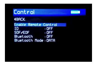
The Control Screen is used to configure the instruments Bluetooth parameters to the user's preference. Pressing the Up and Down buttons navigates through the options, pressing the Enter button selects that option.
