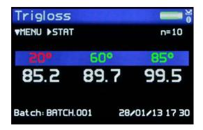
Pressing the Right button in the home screen will access the gloss statistics screen for the current batch for all three angles. Measurements can be taken whilst in this screen and the statistics will be updated.
