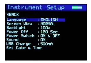
The Instrument Setup screen is used to configure the instruments basic operating environment to the user's preference. Pressing the Up and Down buttons navigates through the options, pressing the Enter button selects that option.
