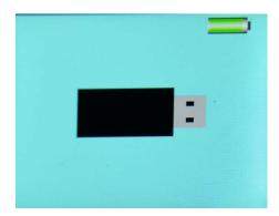
USB Remote Control - Allows control of the Novo-Gloss remotely by sending ASCII commands from a computer or PLC. In this mode the instrument displays "REMOTE CONTROL ACTIVE" on the main measurement screen.
