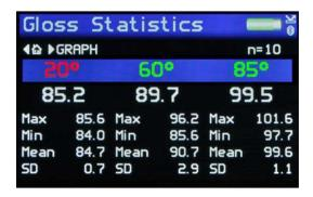
If the pass / fail feature is enabled, the colour of the angle header indicates if the last reading is within the user defined tolerances.
