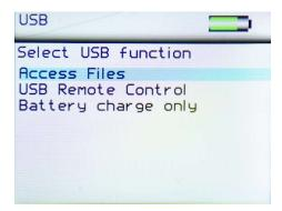
Access Files – Allows access to measurement and configuration files on the instrument. The instrument appears as a USB drive named NG-METER. When selected the display on the instrument shows a USB memory key as shown below –
