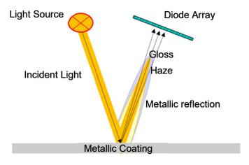
The Novo-Gloss captures compensation information from a region adjacent to the haze measurement angle, this means it can be used on metallic coatings which reflect light directionally
