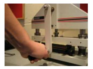
When the handle is perpendicular to the upper and lower chase, the grooves are at their lowest position. •
