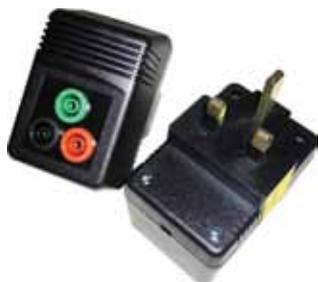
More than just an adaptor, this Test Plug is ideal for electricians and a cost-effective and easy to use means of meeting the NICEIC requirement to confirm the R1 R2 value of a ring main. Establishes that interconnections in the ring do not exist and ensures that the cpc is continuous, indicating the value of (R1 +R2) for the ring.
