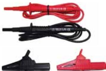
This kit comprises two fused probes at 500mA - 1000V. They include a 50kA fuse on 1.2m double insulated silicone cable, both terminated with a 4mm full safety right angled plug compatible with all standard full safety instrument sockets. Probes and clips included (max 1000V, 500mA fuse). 1000V CAT III.
