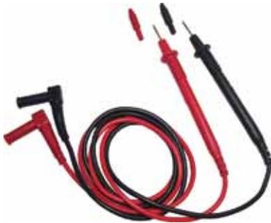
Red and black leads suitable for use with Multimeters and Clamp-on-Ammeters. Shrouded 4mm plugs. Removeable probe cover tips. Double insulated PVC cabling. 1000V CAT III.
