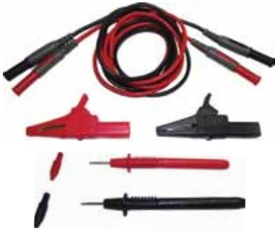
Red and black leads for Multimeters and Clamp-on-Ammeters. Shrouded 4mm plugs. Probes and crocodile clips included. Double insulated PVC cabling. 1000V CAT III.
